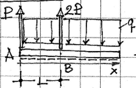
$$N(x) = 0; \quad T(x) = P + 2P - qx \quad \left\{ \begin{array}{l} T_B = T(x)|_{x=L} = 2P \\ T_C = T(x)|_{x=\frac{7L}{2}} = \frac{P}{2} \end{array} \right.$$
