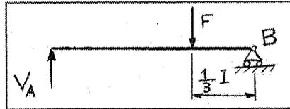
$$V_A l - F \frac{1}{3} l = 0 \quad \text{da cui:} \quad V_A = \frac{1}{3} F = \frac{1}{3} \frac{1}{2} q_0 l = \frac{q_0 l}{6}$$
