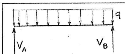
$$\begin{aligned} V_A &= V_B = q l / 2 \\ H_A &= H_B = 0 \end{aligned}$$
